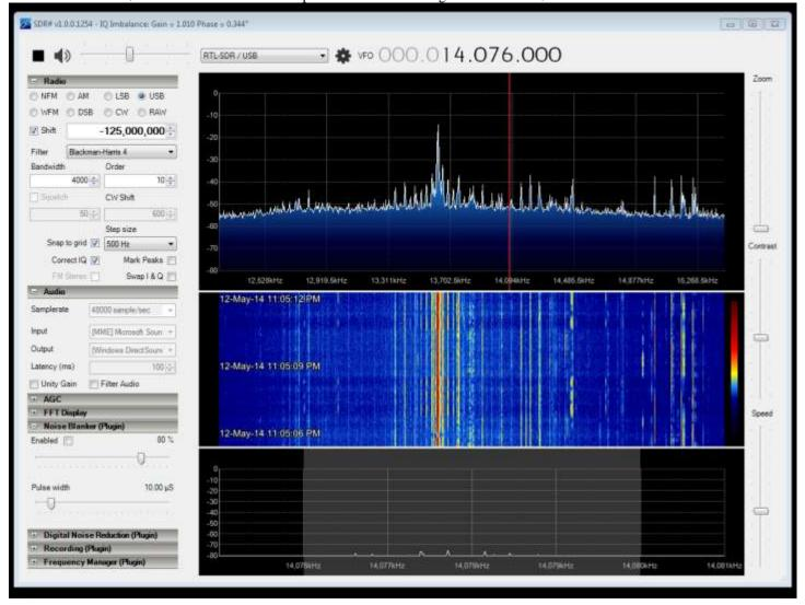
Sample screenshot of SDR#, one of several free "rig-control" apps for the SDR dongle.
